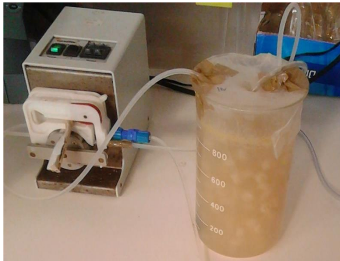
Figure 8 - MBBR in a continuous operation.
