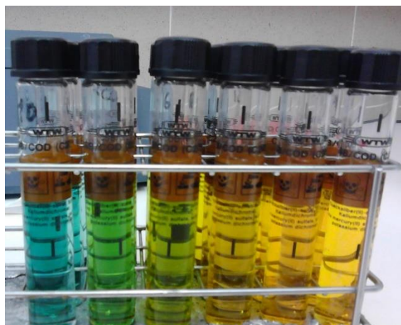
Figure 4 - Vials of calibration curve after reaction.
