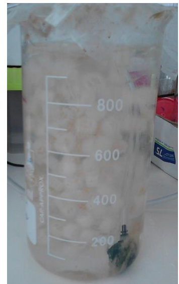
Figure 7 - Lab scale MBBR.
