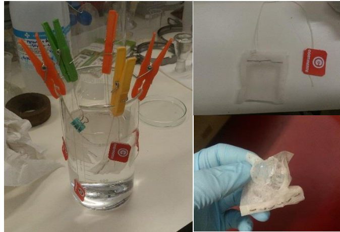
Figure 2.2 – Tea bag method performed.
