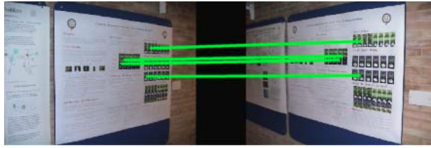
Figure 2.11: Correspondences found between features in very different views of a poster using MSER regions and SIFT descriptors, from [Newman and Ho, 2005]
