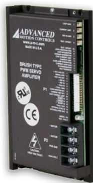
(a) Controlador da Advanced Motion Controls ®, 50A8 [43]
