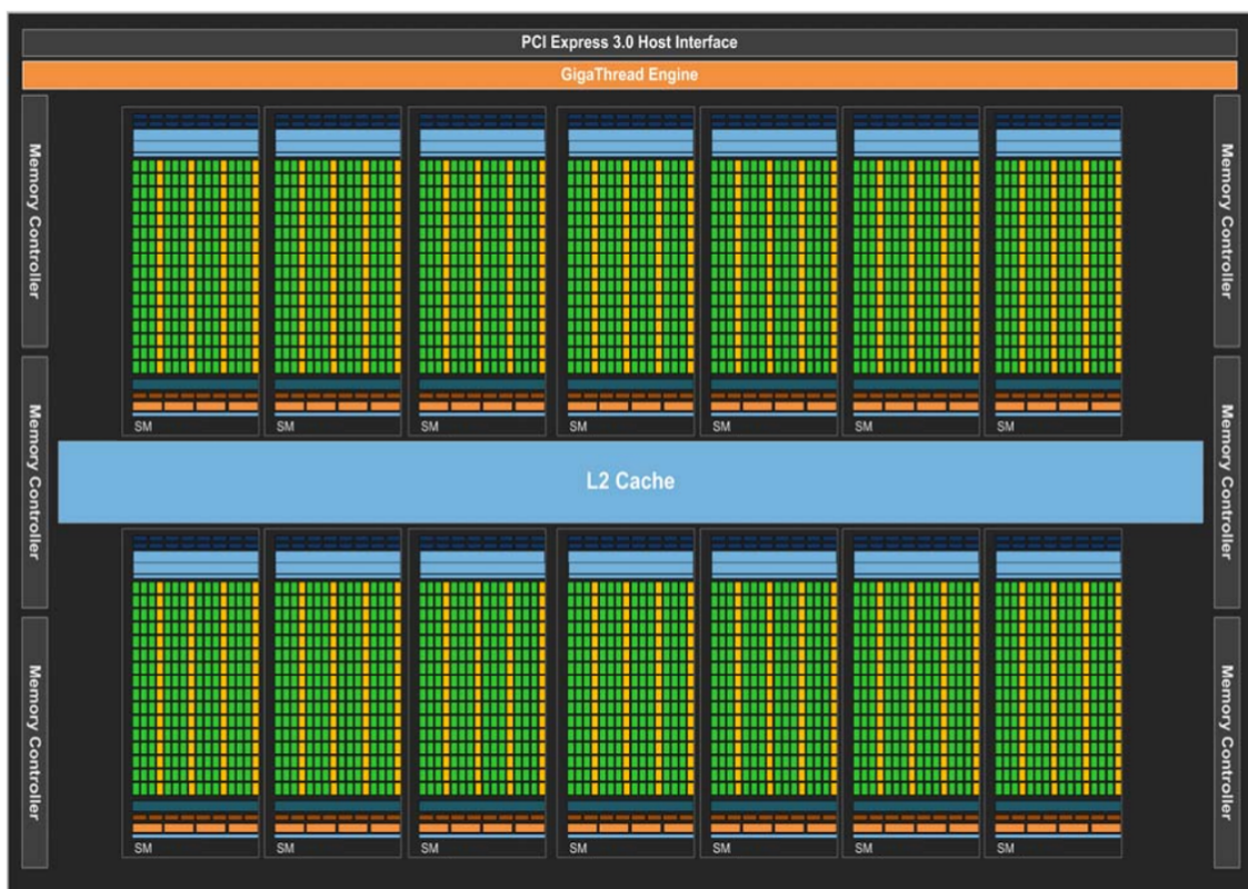
Figure 2.2: Kepler Generic Architecture, 14 Streaming Multiprocessors with the L2 cache [13].
