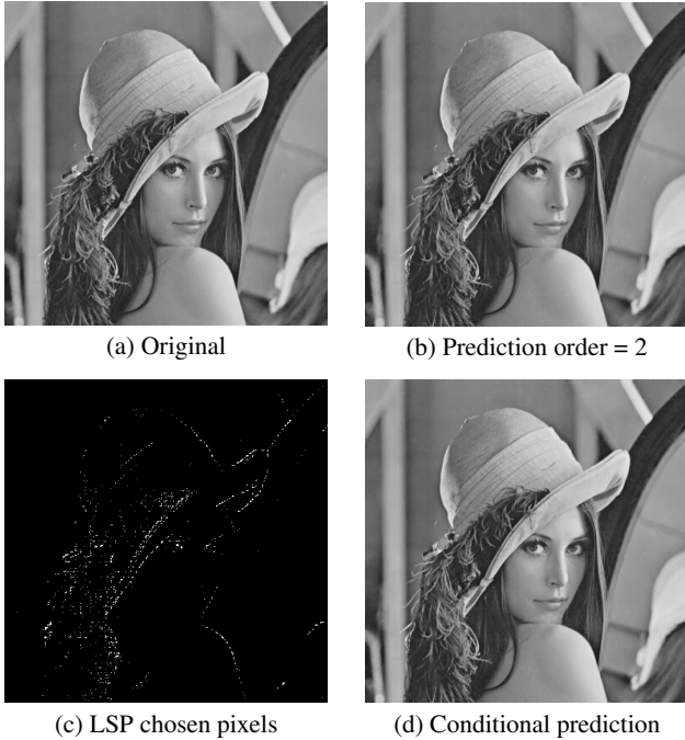
Fig. 3: (a), (b) and (d) correspond to the resulting images of the image coding process for the original image, the prediction order reduction and the conditional prediction, respectively. (c) corresponds to the chosen pixels for LSP prediction
