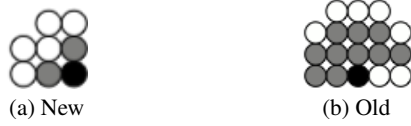
Fig. 2: Left: Original prediction order; Right: Proposed prediction order. The gray pixels are the neighbors considered for the prediction of the black pixel
