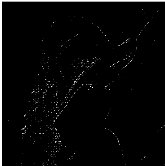
Figure 4.6: The white pixels represent the chosen pixels for LSP prediction. They correspond to edges or near-edges. The offset chosen was 20, i.e., the LSP was applied for pixels that differ in intensity by 20 or more from their 2 neighbors (up and left).
