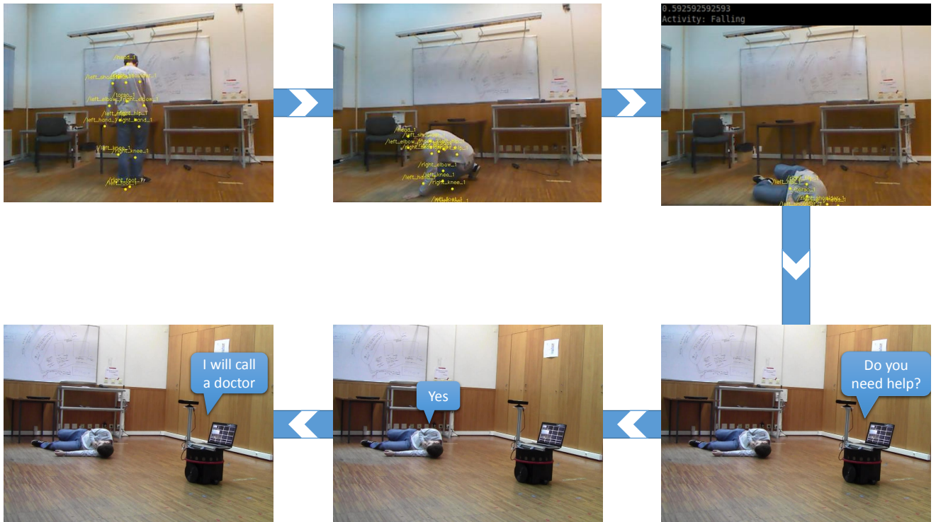
Figure 5.6: Sequence of events on detecting a person falling and reacting.
