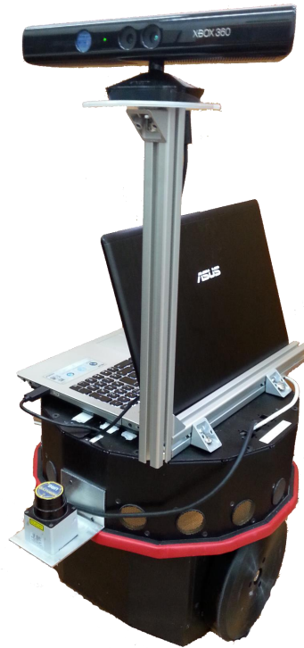
Figure 4.2: The robotic setup used for experiments. It is possible to see the Nomad Scout robot with the elevated structure and Kinect on top of it. On top of the robot is the Asus laptop that was used to control the platform and in the small silver support in the middle of the robot is the Hokuyo URG-04LX Laser Range Finder.
