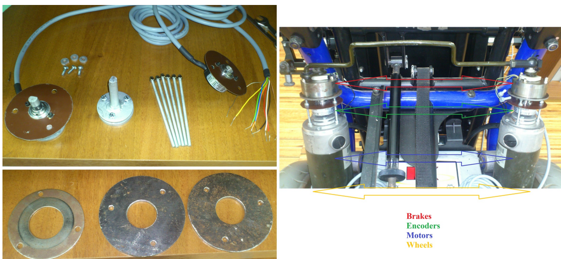
Figure 9.1: On the left, it is presented all the hand-made material to hold the encoders in place while keeping the brakes. On the right, there is a picture taken from below the wheelchair of the final assembly.
