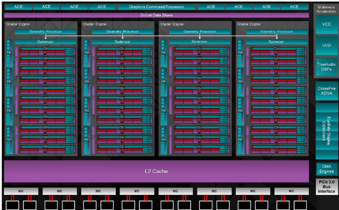
Figure 3.1: The AMD R9 290X (Hawaii) GPU block diagram [2]
