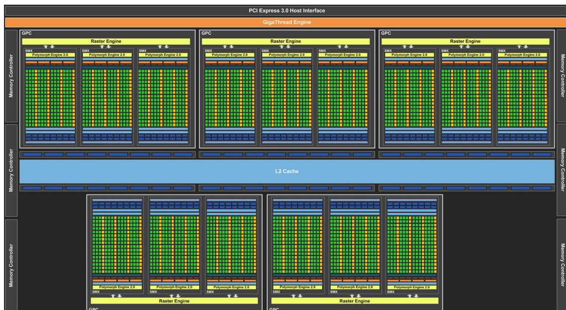
Figure 3.3: The Nvidia GTX Titan (GK110) GPU block diagram [3]
