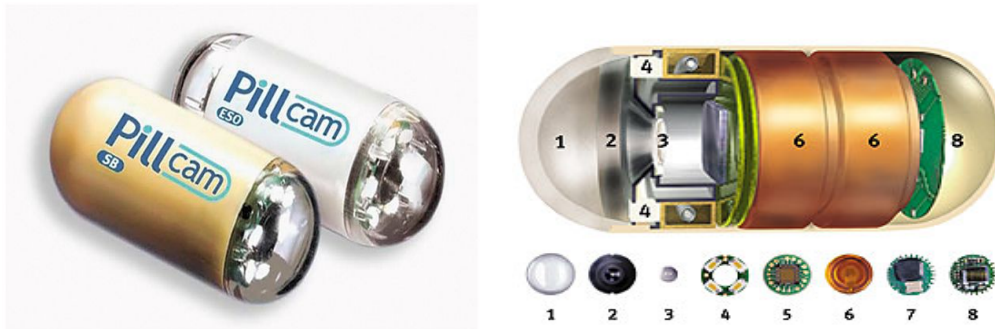
Figure 1.1: Left image: image of the capsule. Right image: view inside the capsule (M2A model features: 1-Optical, Dome 2-Lens Holder, 3-Lens, 4-Illumination LEDs, 5-CMOS (Complementary Metal Oxide Semiconductor), 6-Battery, 7-Transistor ASIC, 8-Antenna)
