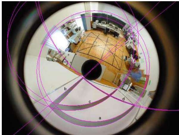
Fig. 13. Estimating the angles between pairs of parallel lines from a paracatadioptric image of those lines.
