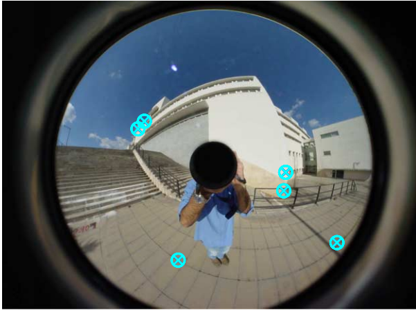
Fig. 12. Estimating the projection of lines in a calibrated paracatadioptric image using two points selected by hand.
