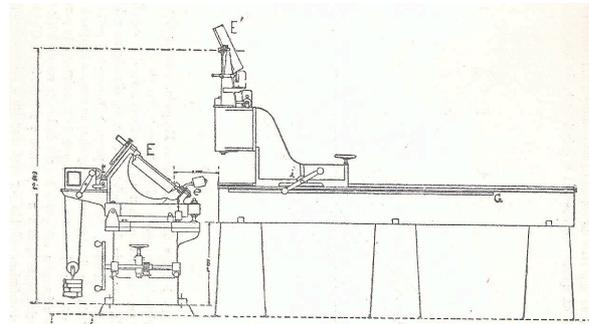
Figure 3: Schematic representation of the coelostat of Coimbra. (Costa Lobo, G.S., 1933b: 453).
