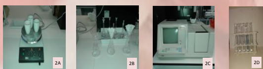
Figure 2- Determination of phosphorus. 2A – Hotplate with crucibles; 2B – Filtration of samples; 2C – Spectrophotometer; 2D – Samples.
