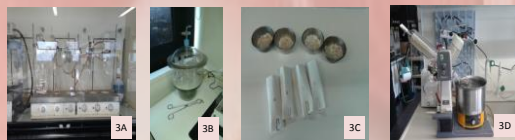
Figure 3. Determination of fat. 3A – Soxhlet extractor; 3B – Desiccator; 3C – Preparation of samples; 3D – Rotary evaporator.
