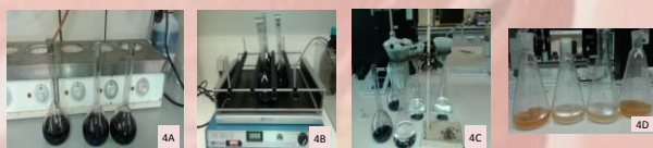
Figure 4- Determination of sodium. 4A – Samples; 4B – Mechanical stirrer with samples; 4C – Filtration of samples; 4D – Samples after titration.
