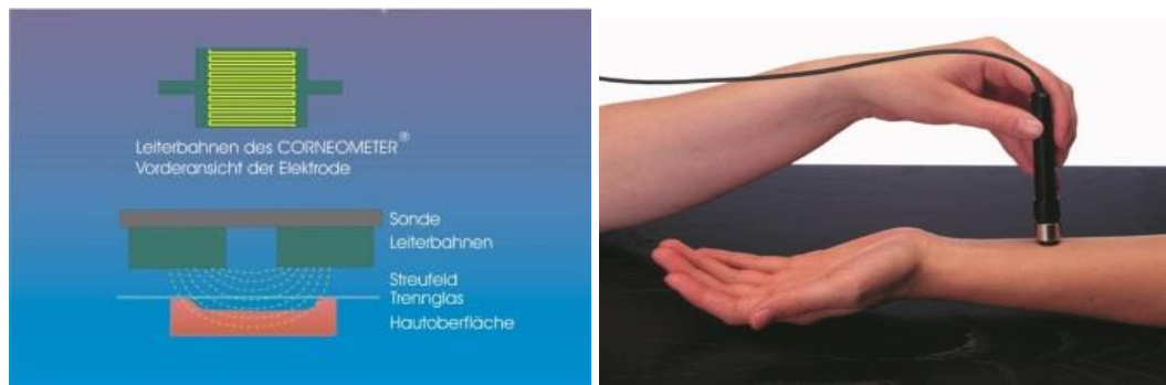
FIGURE 1 - Corneometer® operation principle (with permission from Esther Bász, 2016) (COURAGE-KHAZAKA, 2016)
