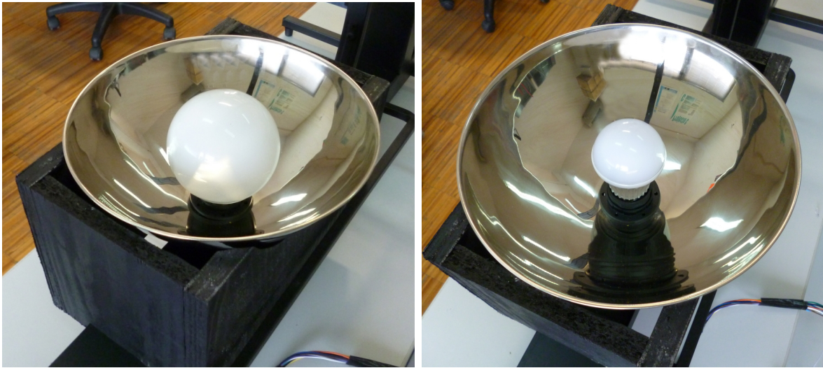
Figure 7.3: Lamp Testing. Left: Compact Fluorescent Lamp (CFL). Right: LED Lamp.
