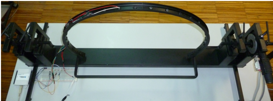
Figure 5.2: Goniophotometer built for the project.
