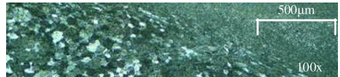
Fig. 5. Optical micrograph showing the microstructure evolution near the advancing side of a S55 weld.
