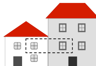
Figure 5. Complex 3D cadastre occurrences in the medieval Coimbra downtown (Portugal): a flat shared by two buildings.
