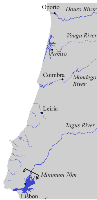
Fig. 6. Lisbon-Oporto rivers' map with the location of the cross-section line defining the upstream limits of the 70 meters bridge height requirement.
