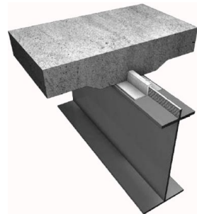
Figure 2.9: Connection with longitudinal embossed steel plates (Papastergiou et al. 2014).
