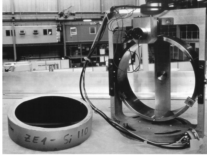
Figure 4.31: Photo of the crystal holder together with a Si(110) crystal at its side. The Si(111) crystal looks similar.
