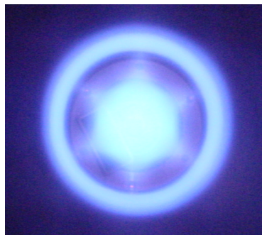
Figure 5.7: Picture of the plasma star inside the ECRIT chamber. The ions follow the field lines of the hexapole (see figure 5.3 on page 103).
