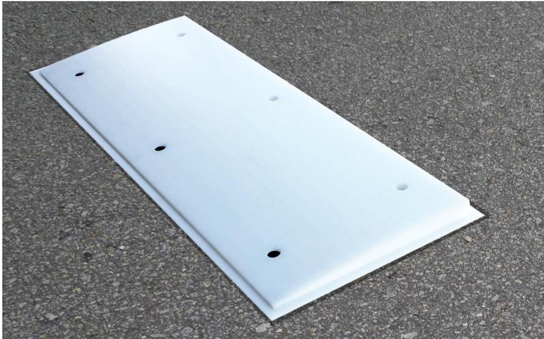
Figure 4.9- Prototype installed in a road pavement.
