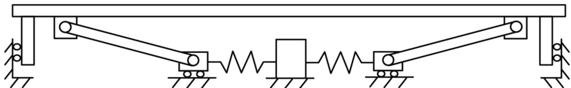
Figure 4.6- SRE with two CTS mechanical systems connected to the surface.
