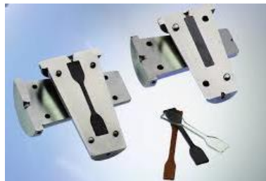
Figure 2.1 – Design of moulds for tensile and flexure specimens
