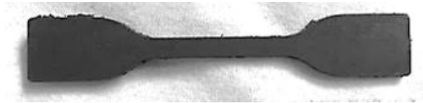
Figure 3.30 –SS 316L “green microspecimen”
