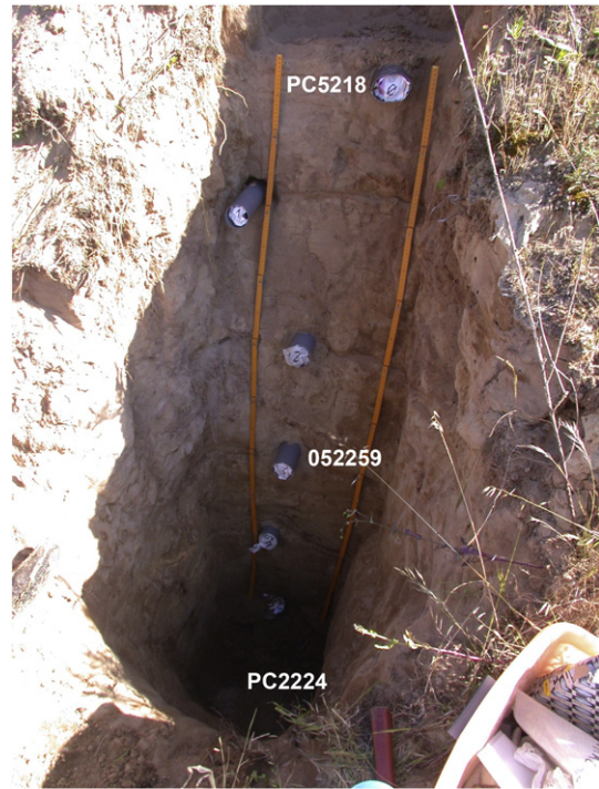
Fig. 15. Outcrop exposing the T5 terrace deposits at Armazéns site, consisting of intertidal medium to fine sands. The codes of the samples selected for luminescence dating can be seen (codes: PC5224 (base of terrace); 052259 (middle of terrace); PC5218 (top of terrace)). The rulers are 2 m long.
