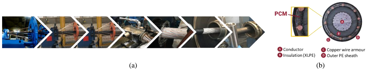
Figure 1. (a) CABELTE's production line with PCM introduction in cable armour; (b) Produced cable with PCM.
