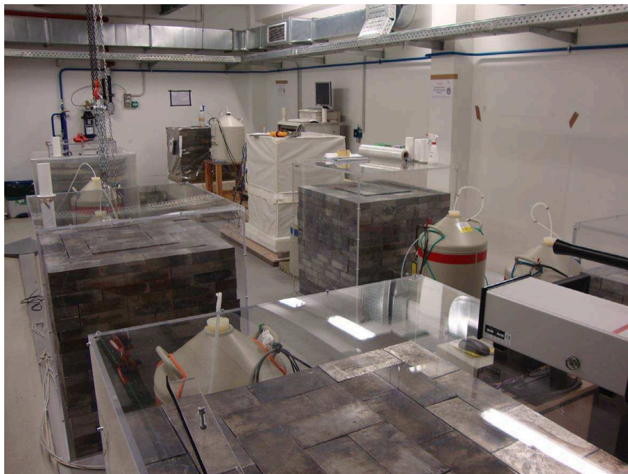
Figure 2. Picture of the Hall C of the LSC where several germanium detectors inside their shieldings are operated for material radiopurity screening (courtesy of LSC). Background counting rates are reported in table 1.
