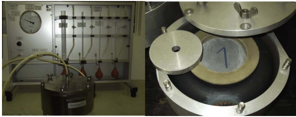
Fig. 3. Gas permeability apparatus and detail of a testing cell.
