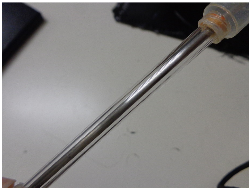
Figure 4.2 Mold used for tube conformation: Stainless steel rod inside of a quartz tube.
