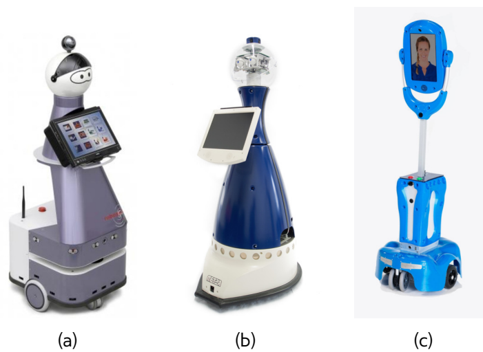
Figure 3.6: Kompai used in DOME0 project (3.6a) and Scitos G5 used in ALIAS project (3.6b) and Giraff/Giraff+ (3.6c).
