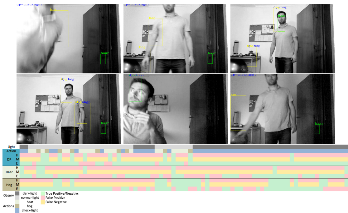
Figure 5.30: Examples of frames from the scenario dataset. From top-left to bottom-right: we see the first two frames and the last, where we have false positives for Haar and HOG algorithms, but the action from the decision process is “Check-light”, which contributes with less errors; the next three frames represent examples of correct detections by the Haar or Hog algorithms and the action selected by the decision process corresponding to most probable algorithm to work under the detected light conditions; at the bottom we summarize the overall results for true positives/negatives in light green, False positives in light red and False negatives in yellow. The first row represents the periods where light conditions were considered normal or dark. The following rows group the results for the decision process, Haar and HOG algorithms.
