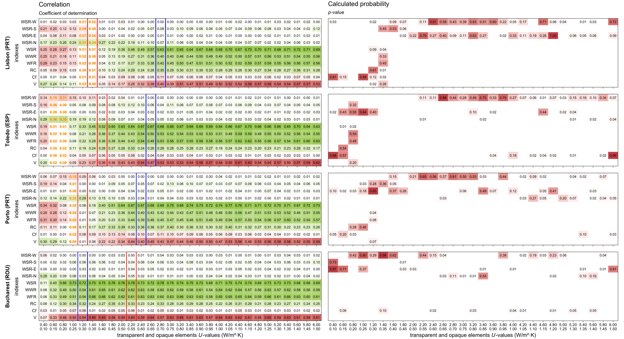
Fig. 7. Correlation of geometry indexes per U -value group per climate location (part 1/2). In the left graphic, green cells show negative correlation and red cells represent positive correlation (maximum reference U -values for opaque and transparent elements are marked as red and blue rectangles, respectively). The orange and bold font U -values columns represent WSR with R^2 \leq 0.02 . On the right graphic, red cells indicate subgroups having p -value above or equal to the threshold of 0.01.
