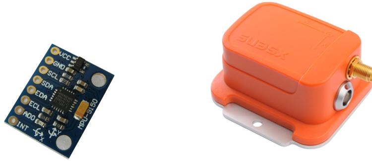
Figure 9: InvenSense MPU-9150 and Xsens MTi-G
