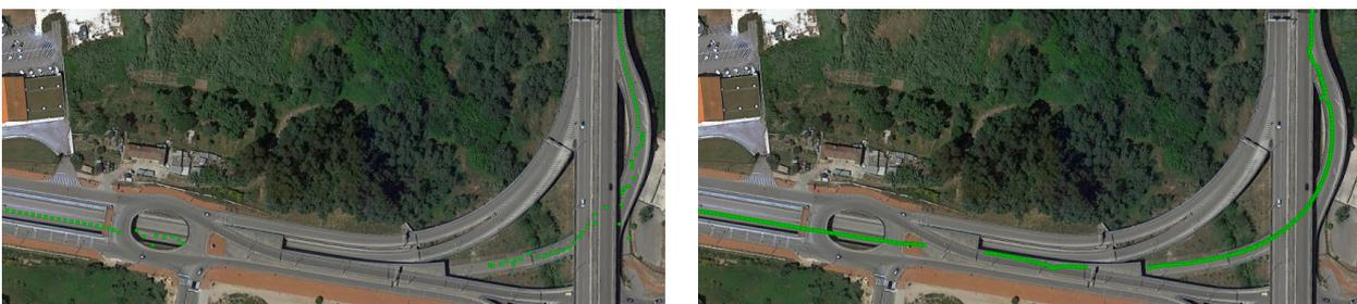
Figure 34: Detailed view from part of the route - 4 - RTK u-blox (left) and RTK Septentrio (right)
