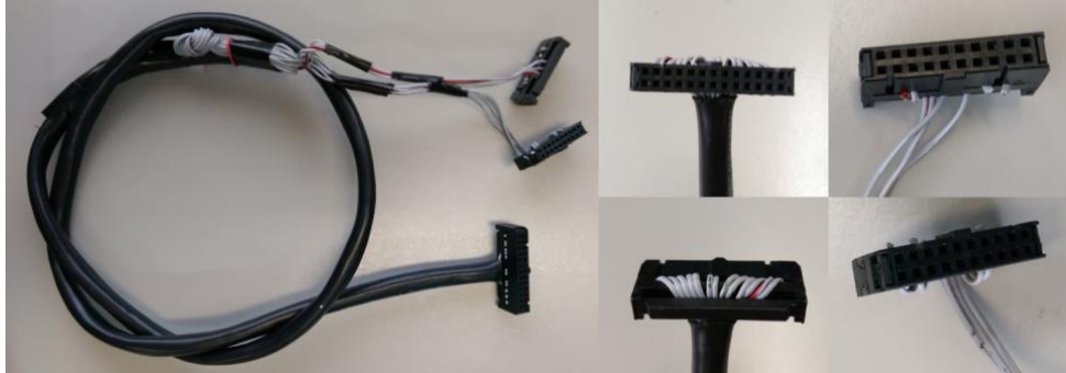
Fig 4.5 Isolate board to inverters boards (Y Cable 26 pins socket to 2x20 pins sockets)
