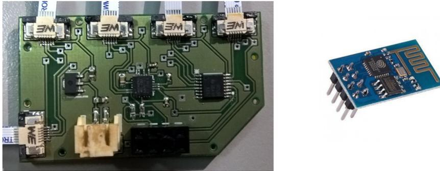
Fig. 4.7 Prototype primary board (left) and ESP8266 ESP-01 board example (right)
