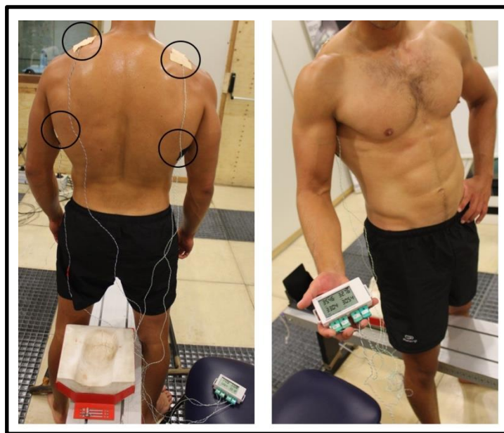
Figure 4 – Thermal sensors application.
