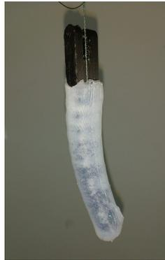
**Figure 3.10:** Soft finger with a silicone layer filled with hydrogel.
