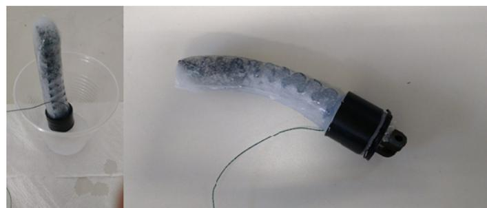
**Figure 3.12:** Little mold cure and removal of the thin perimeter after curing.
