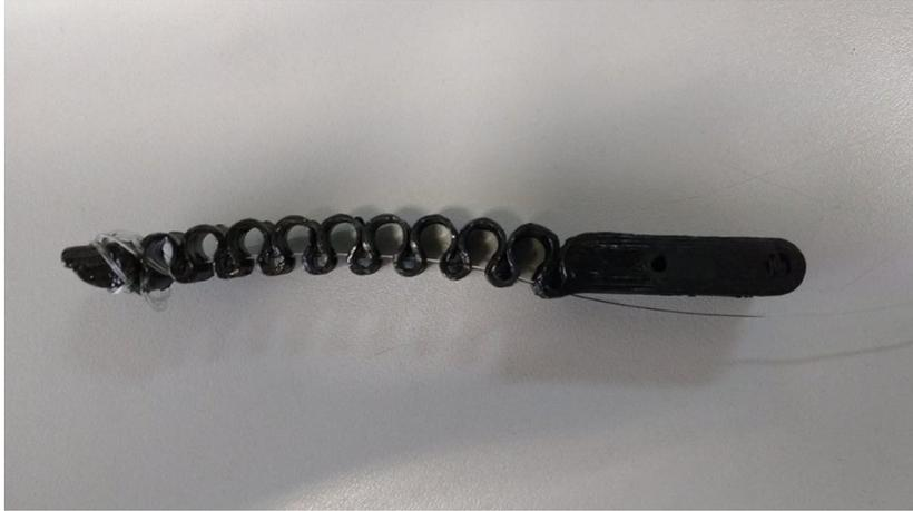
**Figure 3.4:** 3D printed endoskeleton embedded in acetone
