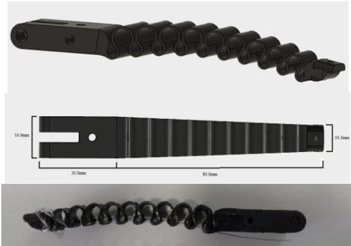
Figure 4- 3D Design of finger endoskeleton and the 3D printed part
