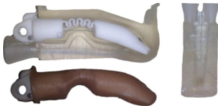
**Figure 3.1:** Previous version of a finger with a 3D printed endoskeleton and a soft skin.
