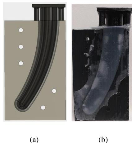
Figure 6- Longitudinal schematic of both molds: (a) 3D design; (b) real picture after curing
