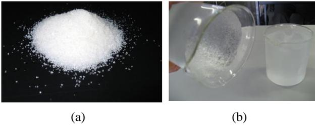
Figure 7- (a) Image of SPA in its pure form; (b) Image of hydrogel created by combining SPA and distilled water
