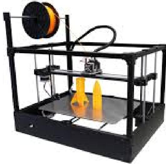
**Figure 2.18:** Example of a FDM Printer [10]
