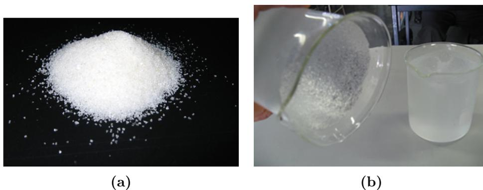
**Figure 2.25:** (a) Sodium polyacrylate in its pure state; (b) Hydrogel made by adding water to sodium polyacrylate.
