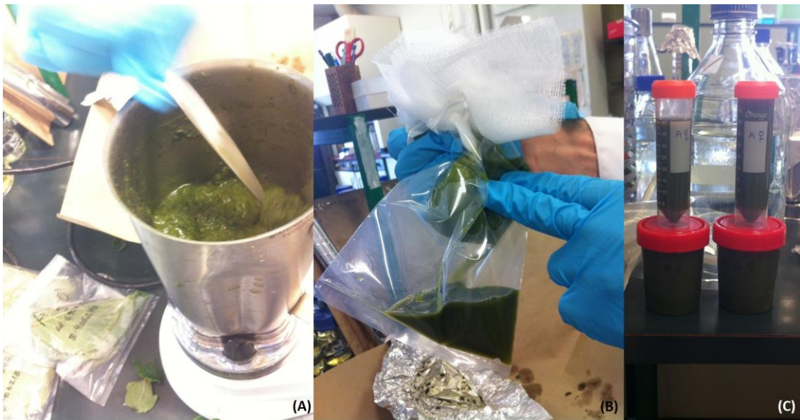
Figure 9 Processing of leaf samples. (A) Grinding of the samples to obtain a homogenate. (B) Filtration of the homogenate for the elimination of vegetable debris. (C) Storage of the sample for further analysis.
