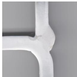
Figure 5.4 – Macro-etched PJP groove weld in matched-width HSS connection (Parker et al , 2013)
