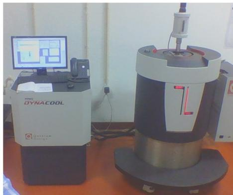
Figure 2.10: PPMS magnetometer of the TAIL facility of the University of Coimbra
