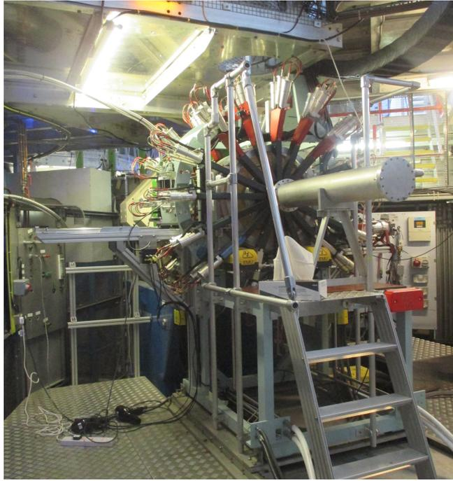
Figure 2.8: Image of the EMU spectrometer, where the positron detectors are clearly visible.
