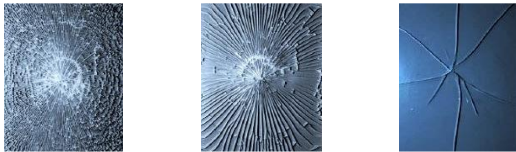
a) Fully-tempered glass b) Heat-strengthened glass c) Annealed glass
