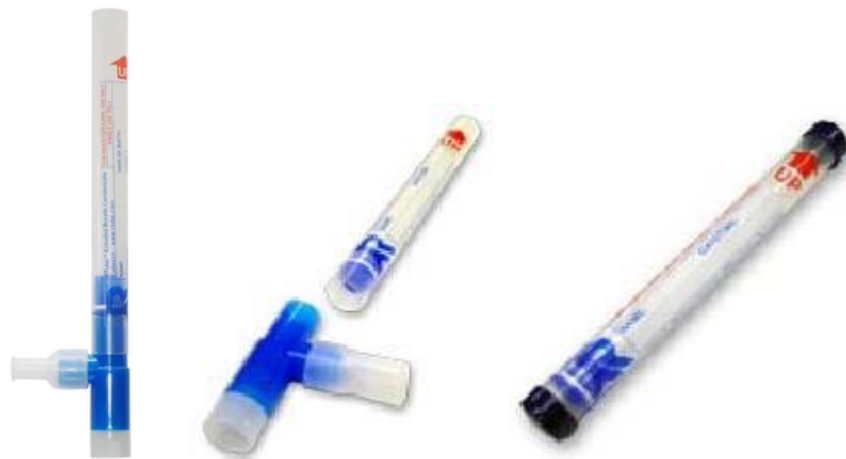
Figure 4: RTube device for exhaled breath condensate (EBC) collection. RTube disposable collection system consists of a unidirectional valve crafted from silicone rubber, a large polypropylene Tee section separating the saliva from the exhaled air; and a polypropylene collecting tube that is cooled by an aluminum sleeve placed around it. (RTube™ -Respiratory Research)
