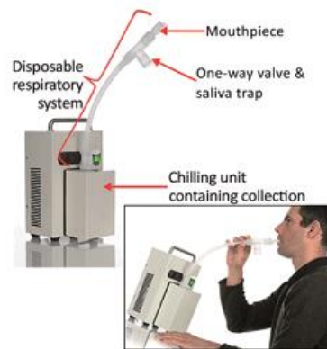
Figure 5: TurboDECCS device for exhaled breath condensate (EBC) collection is comprised of a portable Turbo Unit and a disposable DECCS collection system. DECCS is composed by a mouthpiece, a one-way aspiration valve, a tube, and a collection cell inserted in a Peltier-type electrical cooling system (Leese, Morton, Gardiner, & Carolan, 2016).
