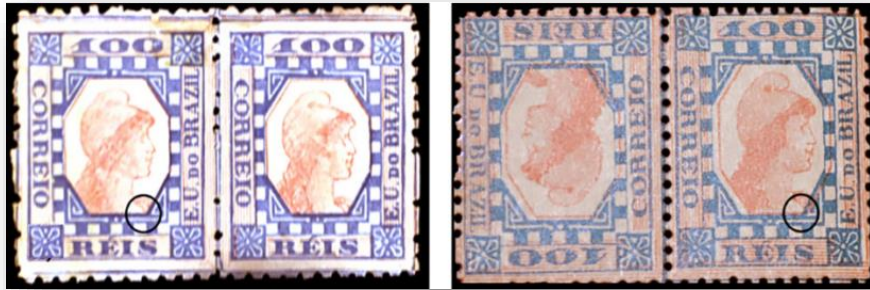
Figure 1.4.1 – An authentic ( Left ) and suspect of counterfeiting ( Right ) postage stamps. The area with a circle indicates the analyzed area (from ref. 16 ).
