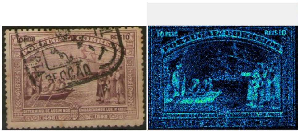
Figure 3.1.4 – Mapping of 150_1898_Rep2 postage stamp for Pb. Acquisition conditions: current at 1000 \mu A; collimator at 0.2x0.2mm; pixel size 70 \mu m/pixel; time per pixel 50,00 ms; voltage at 50kV; filter: for Pb.
