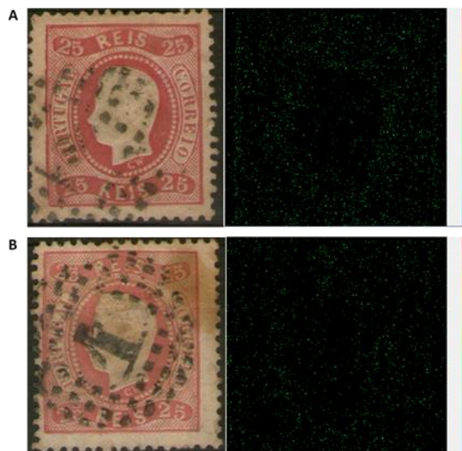
Figure 3.1.3 – Mapping of (A) 30_1867_Rep1 and (B) 30_1867_Rep3 postage stamps for Hg. Acquisition conditions: current at 1000 \mu A; collimator at 0.2x0.2mm; pixel size 60 \mu m/pixel; time per pixel 50,00 ms; voltage at 50kV; filter: for Hg.
