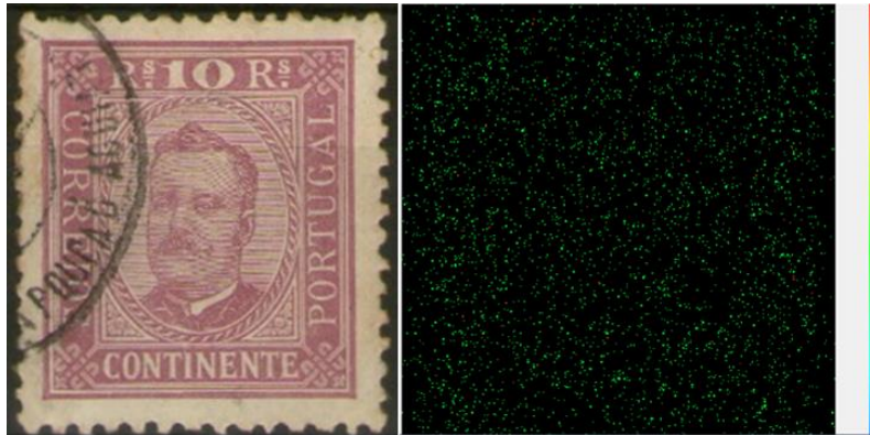
Figure A1.2 – Mapping of 69_1892-94 postage stamp for As. Acquisition conditions: current at 1000 \mu A; collimator at 0.2x0.2mm; pixel size 70 \mu m/pixel; time per pixel 50,00 ms; voltage at 50kV; filter: for Pb.
