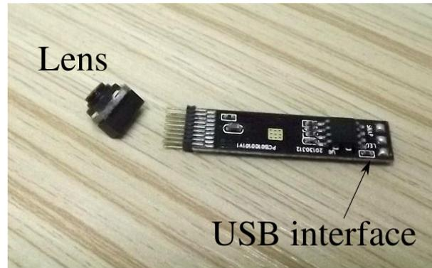
Figure 2.5: Endoscopy camera used
