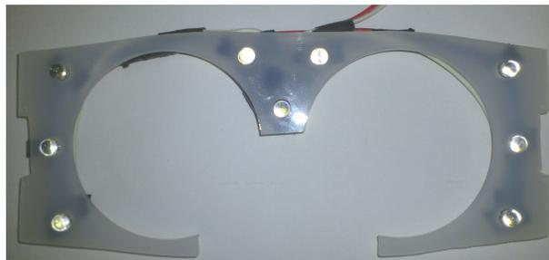
Figure 2.6: Acrylic plate with IR LEDs
