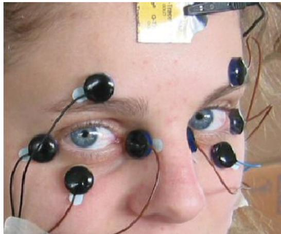
Figure 1.5: Electro-OculoGraphy system [17]
