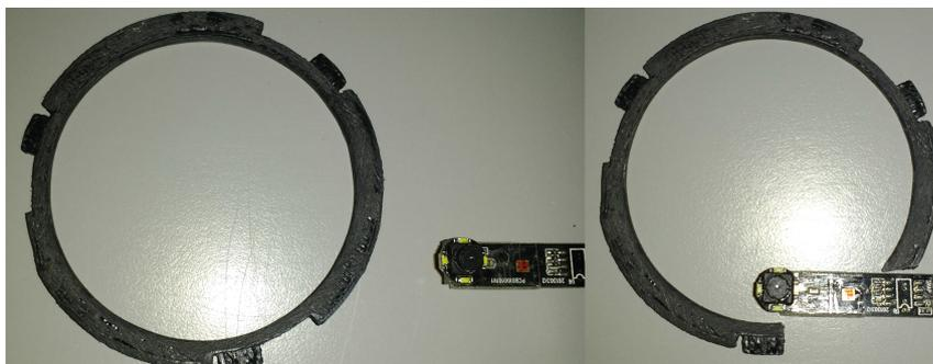
Figure A.3: Bottom part (right) before/after the cut is made to fit the camera
