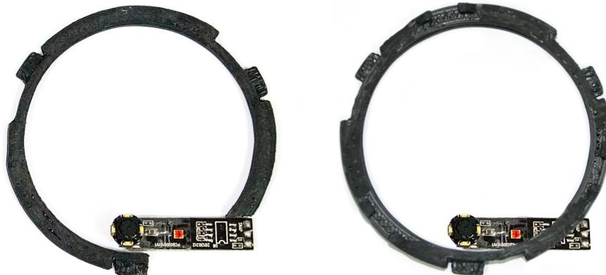
Figure 2.11: Detail of the spacer showing the camera positioning
