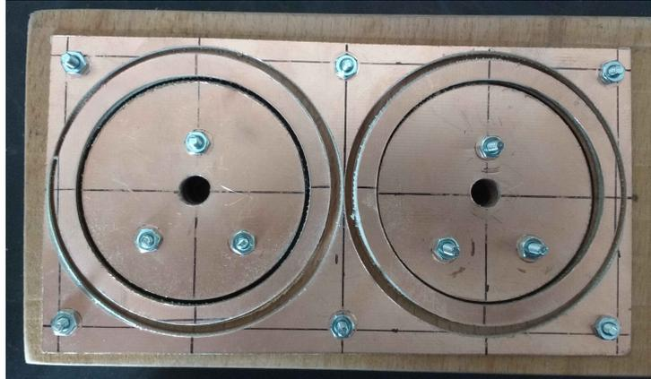
Figure B.3: Jig to cut the PCB rings
