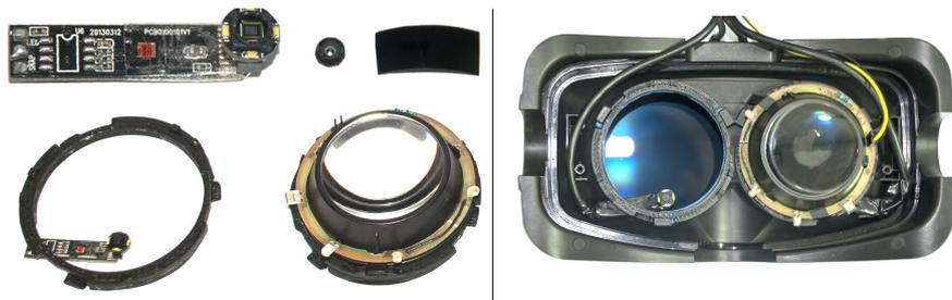
**Fig. 1.** Left: Camera board and sensor with 90 degrees bent connections; Lens; IR filter (film); Lens on spacer with IR ring; Spacer with camera below; Right: Oculus Rift DK2 with left lens out, showing spacer and camera installed; on the right side we can see the illumination ring in mounted on the respective lens.
