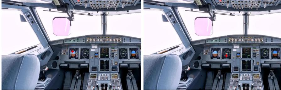
**Fig. 3.** Example of the output of eye tracker (red cross) mapped onto a plane cockpit shown to the user.
