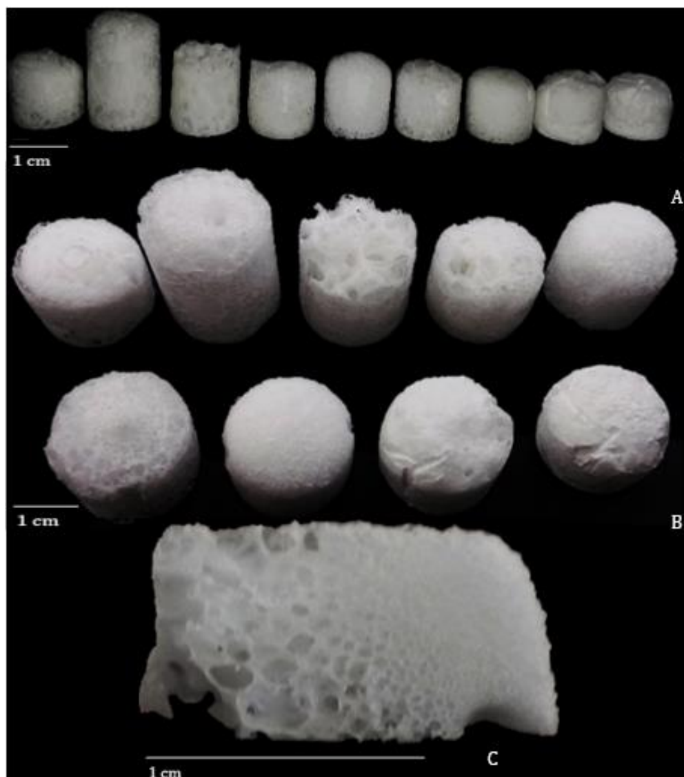
Figure D.1 – Macroscopic visualization of SFM processed samples, side view (A) and top view (B). On A, from left to right: A84, A98, M98, T98, A74, M74, T74, A98+SNPs, A74+SNPs. On B: above, from the left to right: A84, A98, M98, T98, A74. Down, from the left to right: M74, T74, A98+SNPs and A74+SNPs. In C, slice cut top-to-bottom of sample A74+SNPs: PCL 3 sizes + 74 molar % of GF + 17 wt.% SBA-15. The left side corresponds to the bottom and the right side to the top. Scale bar: 1 cm.
