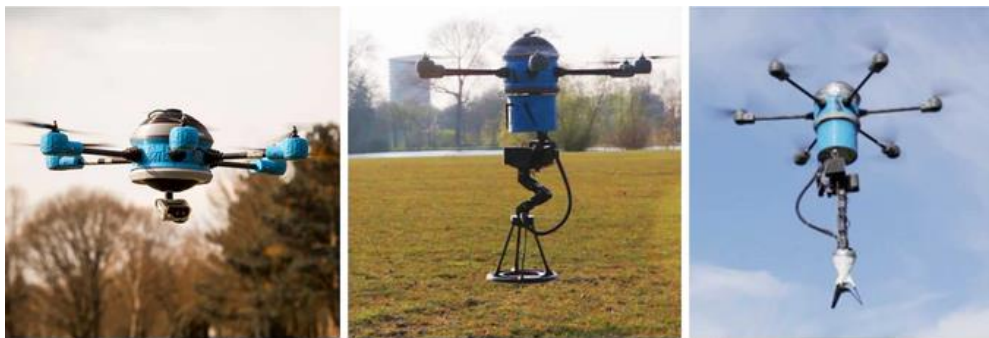
Figure 2.5 - Mine Kafon Drone mapping, detecting and detonating steps respectively [21].
