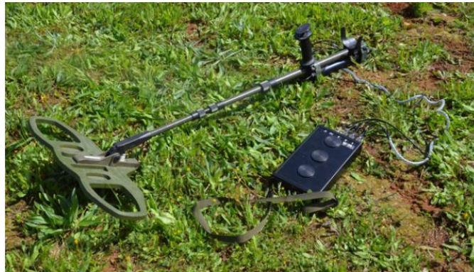
Figure 2.10 - The original metal detector, before it was mounted to the robotic arm [25].
