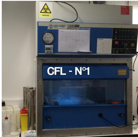
**Figure 10. Vertical laminar flow chamber from Gelaire**
