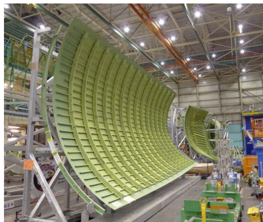
Figure 1.3: Fuselage stiffened curved panel of a Boeing 777 [10]
