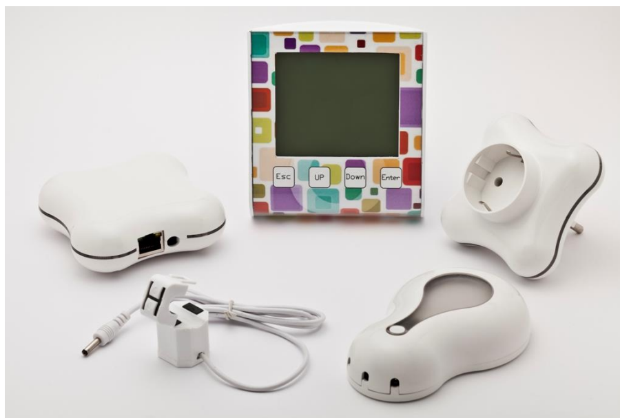
Figura 3.3 – Concentrador, sensor, transmissor, monitor e tomada inteligente. (Martins, 2013)
