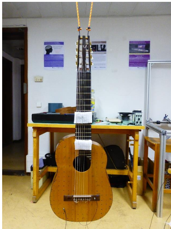
Figure 20 Free-boundary guitar set-up
