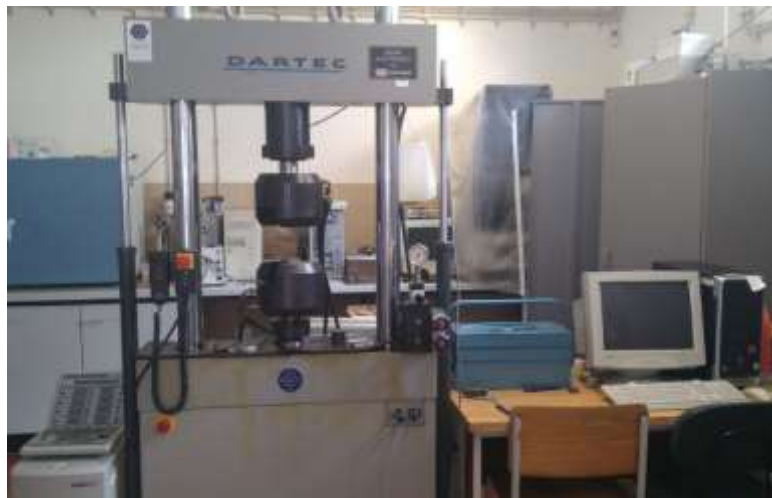
Figure 3.3: DARTEC servo-hydraulic and its constituents (control panel and computer, from left to right).
