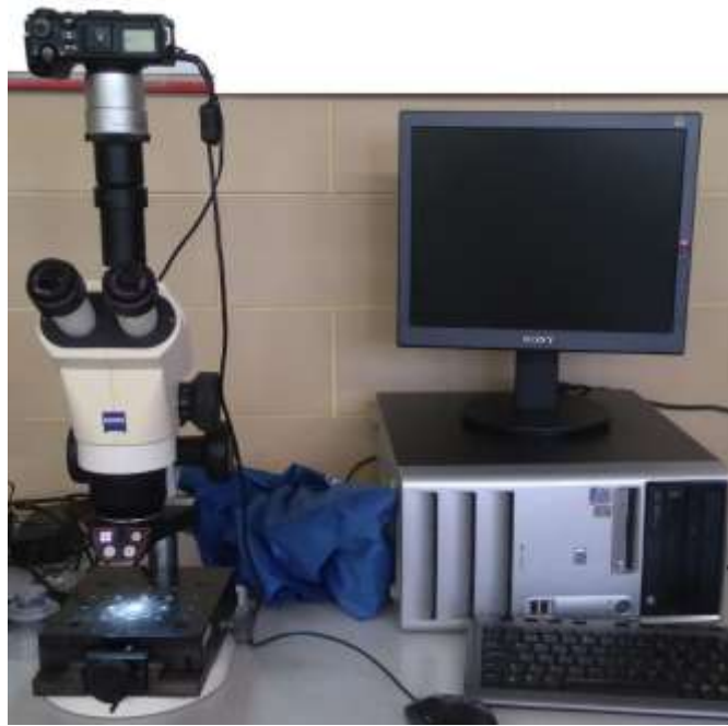
Figure 3.5: Equipment used to perform the OM tests (from left to right: microscope with the camera attached, computer).
