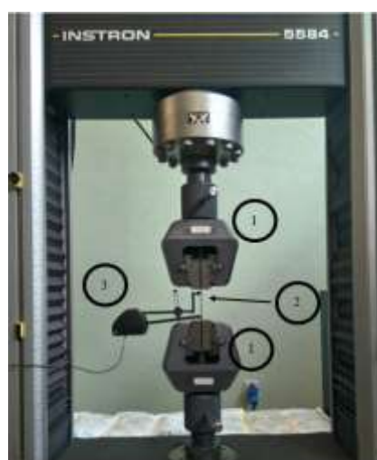
Figure 3.2: INSTRON 5584 servo-hydraulic machine (1- Grapples; 2- Specimen; 3- Mechanical extensometer).
