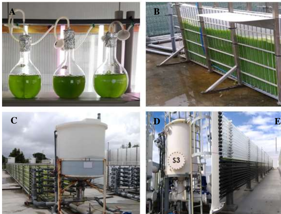
Figure 5 - Pictures from ALGAFARM unit: laboratory air-lifts 5 L (A); GWP 125 L (B); PBR 2500L (C); PBR 10000L (D and E).
