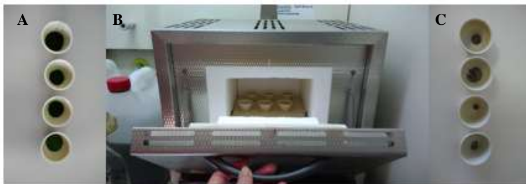
Figure 6 - A: Ceramic cup with biomass; B: Furnace with the samples inside; C: Ceramic cups with resulting ashes.
