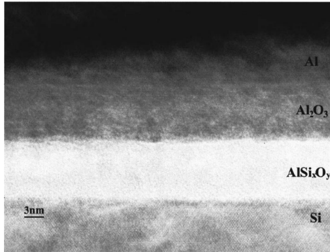
Figure 1.3: The low- \kappa interfacial layer for a high- \kappa dielectric, \text{Al}_2\text{O}_3 , from [WWA01].
