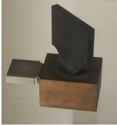
Figure 2.7: Graphite target used at ISIS facilities in England with dimensions 50 \times 50 \times 7 mm.
